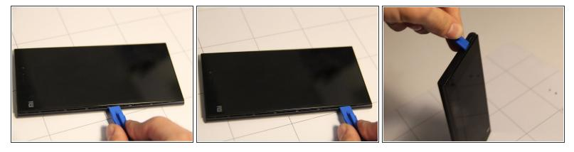
• Once the pry tool has been inserted into the phone, slide it around the perimeter of the phone while gently lifting until the screen panel and back panel of the phone separate.
