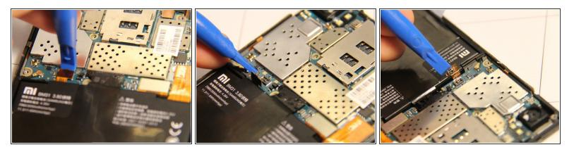
Using a spudger, remove the small ribbon cable that is connected to the battery.
