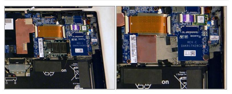
Pull the SSD towards the right and slightly up, removing it from the back assembly.
