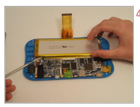
Once this is done start to pry the battery away from the device carefully. It helps to start at the corners and move inward.
