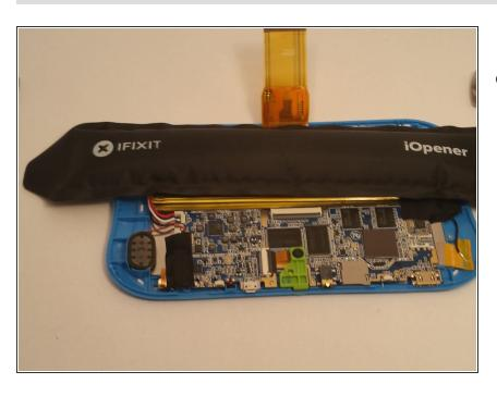
Next you must heat up the battery to help weaken the adhesive connecting the battery to the device.
