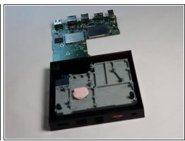
Place your finger on the short edge of the motherboard and lift it to separate it from the plastic case.
