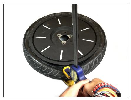
Use the clamp to squeeze the rubber of the tire until the tire pops off of the rim. Repeat this process until the whole tire is popped off of the rim.
