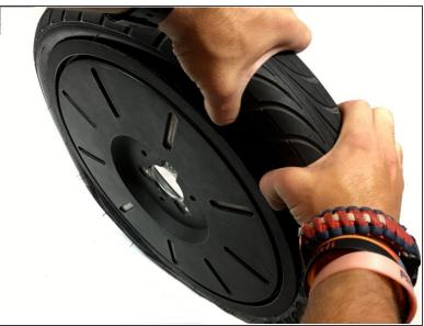
• Make sure the tire isn't all the way on the rim, otherwise the last quarter of the tire will be almost impossible to pry back into place. To make sure the tire is not on the rim, repeat what was done in step three when the tire was squished off of the rim.
