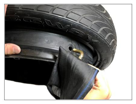
When you are sure you have the correct inner tube, take the nub of the new inner tube and put it back into the hole of the rim that the old inner tube nub was removed from previously.
