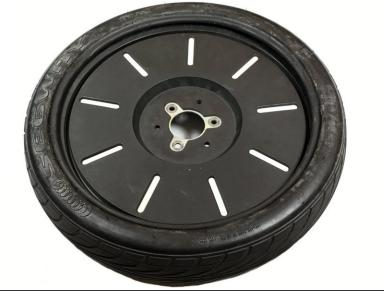
Continue pulling the rubber over the rim until the edge of the rubber is visible all the way around the tire.
