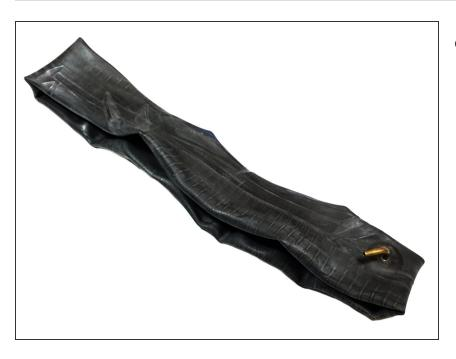
Take the new inner tube for the Segway and make sure it's deflated and is the right model number for your Segway.
