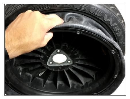
Wrap the new inner tube around the rim.
