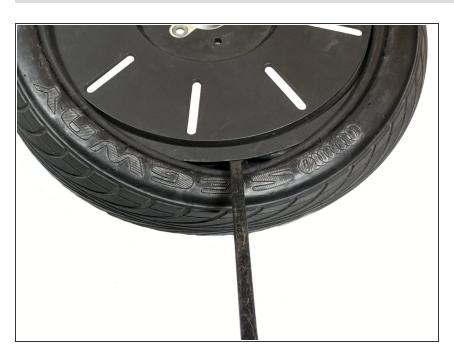
Use the persuasion bar to begin pulling the rubber back over the rim of the tire. When you pull the rubber back over the tire, push the persuasion bar away from you and towards the other side of the tire to put the rubber of the tire back onto the rim.
