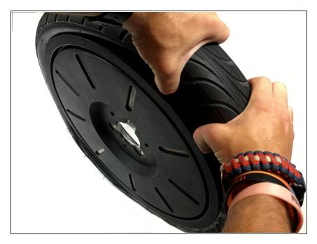
Use your hands to squish the tire all the way around the sides to make sure the tire is off the Segway rim completely.
