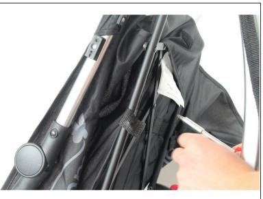
Remove the two silver 12.7 mm #01 screws (1 on each side) holding the back of the seat to the frame.
