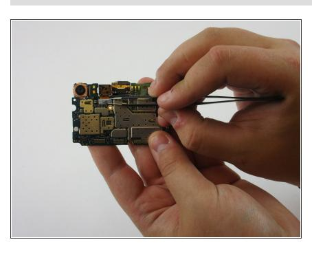
The front camera is attached to the motherboard by a ribbon, use tweezers to detach it from the motherboard. To reassemble your device, follow these instructions in reverse order.
