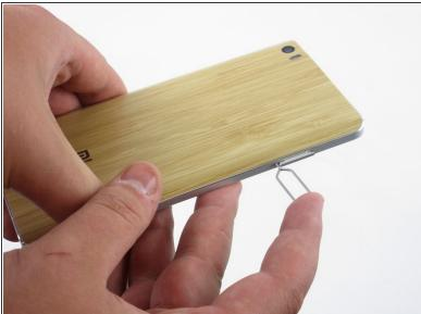
Use the Dual SIM SD card removal tool (or use a paper clip) and insert it into the slot hole until the tray pops out.
