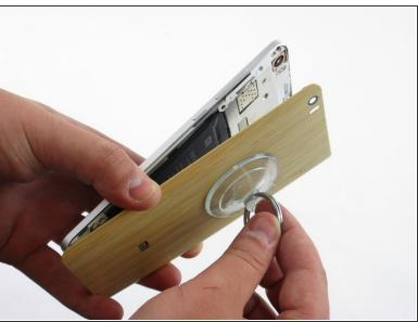
Use your suction cup to grip the back of the phone. Once the suction cup is secure, pull back with moderate force and the back plate should snap free.
