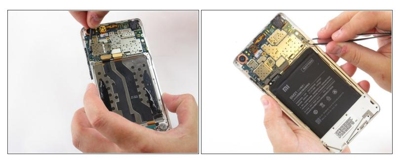
Use tweezers to detach the small ribbon on the left side located near the volume buttons as well as the microphone cord located on the right side along the frame.
