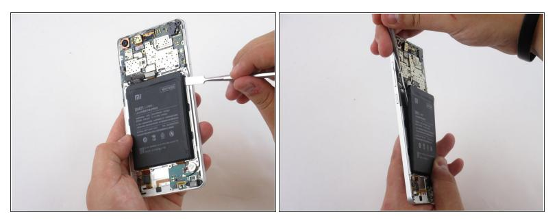
Insert a nylon or metal spudger underneath the battery at any point. Then slide the spudger around all the edges to loosen it. The battery can now be easily lifted out of the frame.
