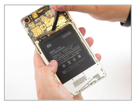
Use a plastic spudger to detach the remaining ribbon from the motherboard.
