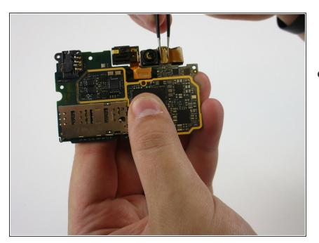
Use tweezers to slide the ribbon to the right out of the insert as shown in the image.
