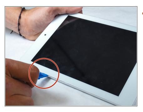
Pry the back case off using the blue Plastic Opening Tools. Work one along the seem until you can get your fingers under to pull it apart.
