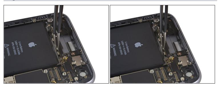
• Deroute the upper left cellular antenna cable from the first logic board clip by nudging it out from under the clip, towards the battery.
