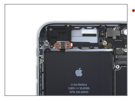
• Remove the two 2.7 mm Phillips screws securing the audio control cable bracket to the logic board.
