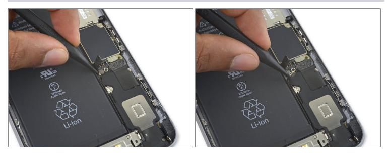
• Disconnect the antenna cable by prying it up from the logic board.
