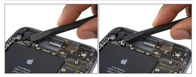
• Disconnect the audio control cable by prying its connector straight up from its socket on the logic board.
