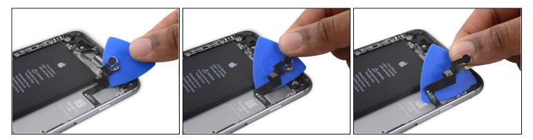
• Slide an opening pick underneath the power button flex cable to pry the cable off the rear case.
