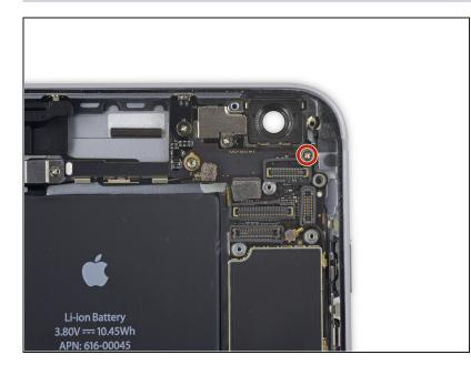
• Remove the single 1.4 mm Phillips screw holding the NFC bracket in place.
