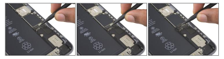
• Use a spudger or a clean fingernail to disconnect the battery connector by prying it straight up off the logic board.
