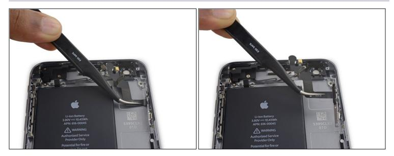
• Remove the power button flex cable.
