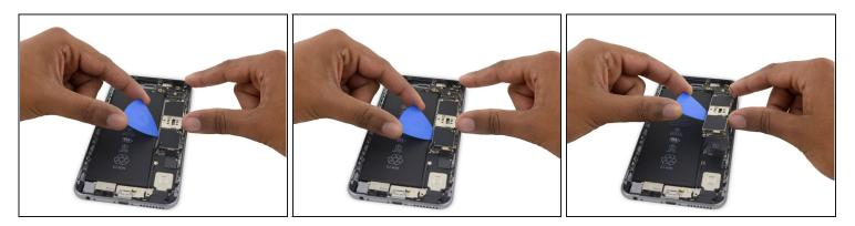
• Carefully raise—but do **not** remove—the logic board, lifting it from the bottom edge nearest the Lightning connector.
