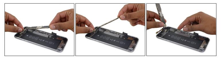
• Tip the logic board up to a vertical position to expose the single antenna connector on the underside, near the top edge of the board.
