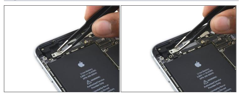
• Remove the audio control cable bracket.
