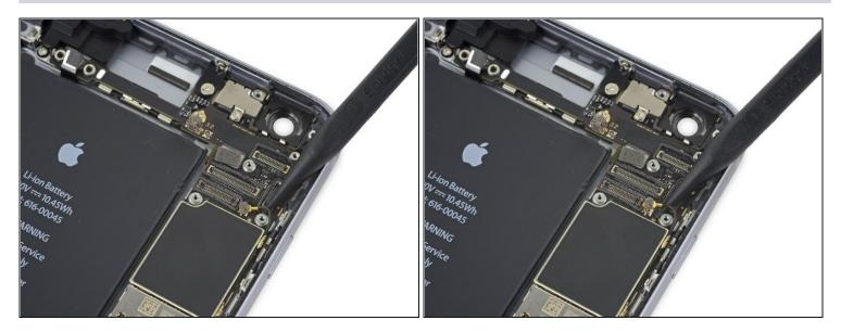
• Disconnect the Wi-Fi diversity antenna cable by prying its connector up from the logic board.
