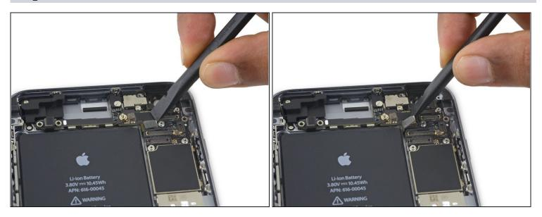
• Disconnect the power button flex cable from its socket on the logic board.
