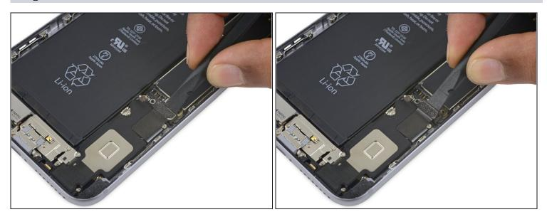
• Use the flat end of a spudger to disconnect the Lightning connector flex cable from the logic board.
