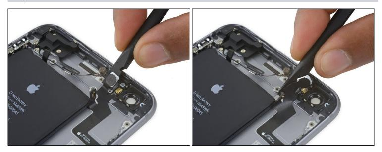
• Use the flat end of a spudger to peel the power button flex cable off the rear case.
