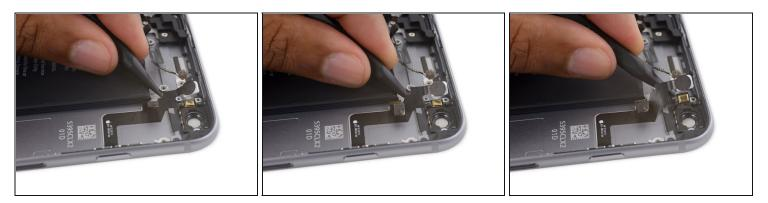
• Insert the tip of a spudger underneath the microphone portion of the flex cable and gently pry it off of the rear case.
