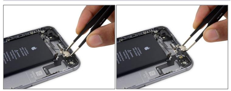
• Remove the flash/microphone bracket.
