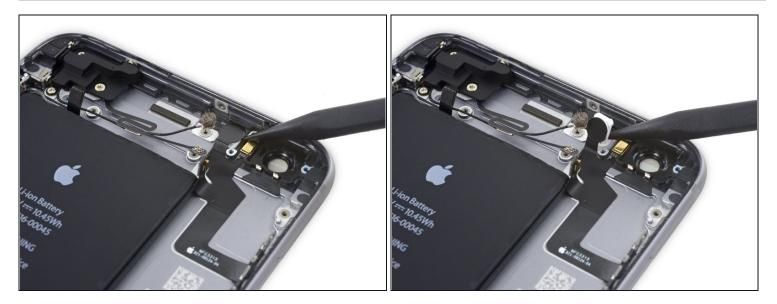
• Use the pointed end of a spudger to lift the flash out of its housing in the rear case.
