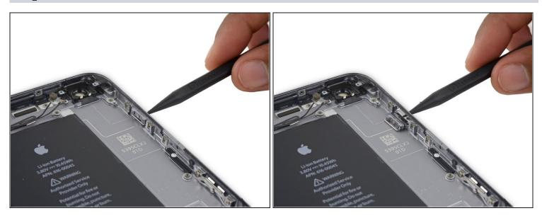
• Gently nudge the power button cover out of its slot in the rear case.
