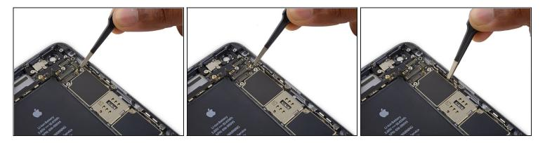
• Deroute the antenna cable from the two clips on the right edge of the logic board.
