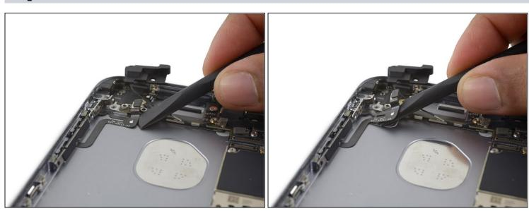
• Use the flat end of a spudger to peel the volume control flex cable off the rear case.
