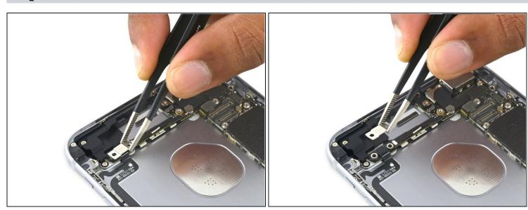
• Remove the audio control cable bracket.
