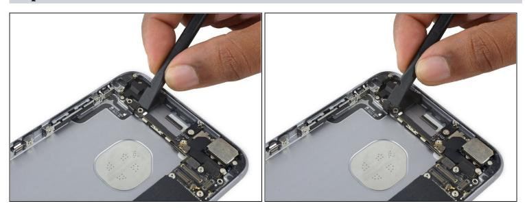
• Disconnect the audio control flex cable from its socket on the logic board.
