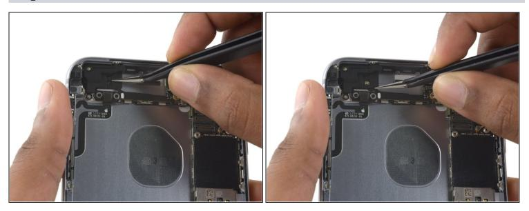
• Remove the circular sticker covering the third screw securing the cellular antenna to the rear case.
