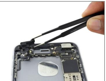
• Lift, but do not remove, the cellular antenna to reveal the third screw securing the audio control cable to the rear case.
