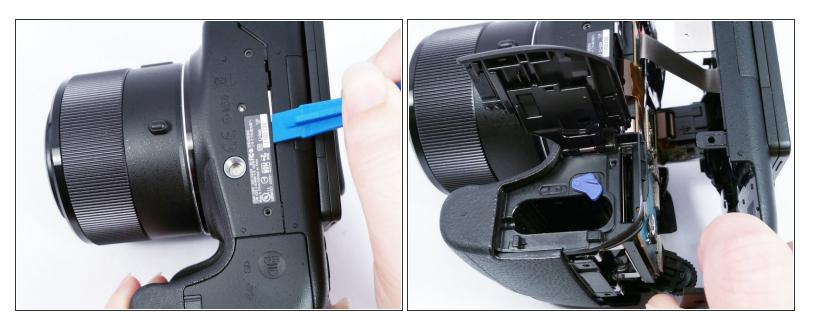
Using a plastic opening tool, separate the plastic camera housing.
