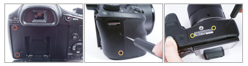
Make sure to remove the battery before disassembly to prevent electrocution.
