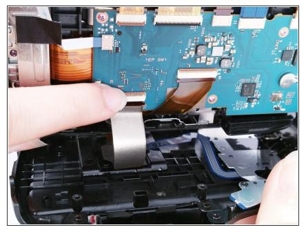
• Disconnect the ribbon wire attaching the screen to the camera.
