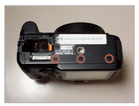
Remove the three black 4 mm JIS #0 screws on the bottom of the camera.
