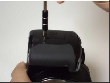
• Remove the two black 6 mm Phillips screws from the right side of the camera.
