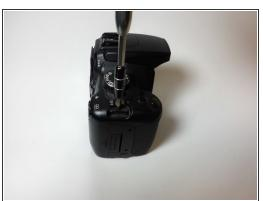
• Remove the two black 4 mm Phillips screws on each side of the camera under the strap hooks.
