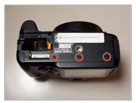
Remove the three black 4 mm JIS #0 screws on the bottom of the camera.
