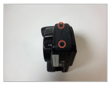
Remove the two black 4 mm Phillips head screws on the side of the camera opposite to the hand grip.
