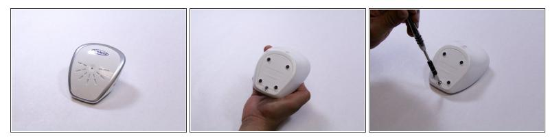
• Remove the 9mm screw from the battery cover of the nursery unit using a Phillips #1 tip screwdriver.
