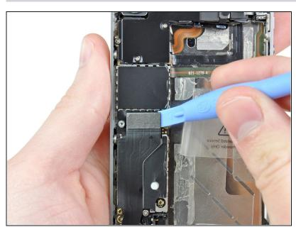
Use the edge of a plastic opening tool to pry the dock cable up from its socket on the logic board.
