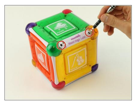
Remove two 6 mm Phillips #2 on either side of the On/Off Plate.
