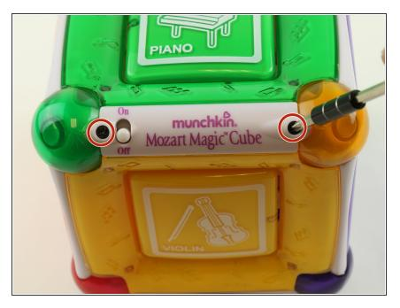
Lastly, re-insert the battery cartridge followed by the face plate, and then tighten the screws.
