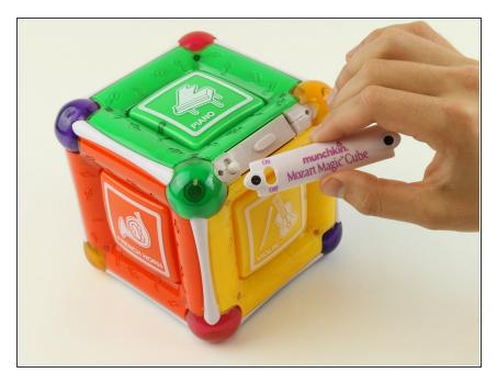
Carefully remove the battery door.
