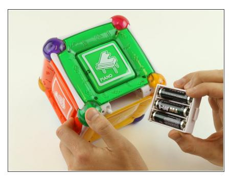
Gently pull out battery cartridge, and replace the batteries.
