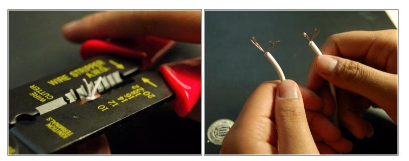
• Strip the wires using wire strippers.
