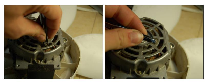
• Clean out the dust from the blades and motor using tweezers.
