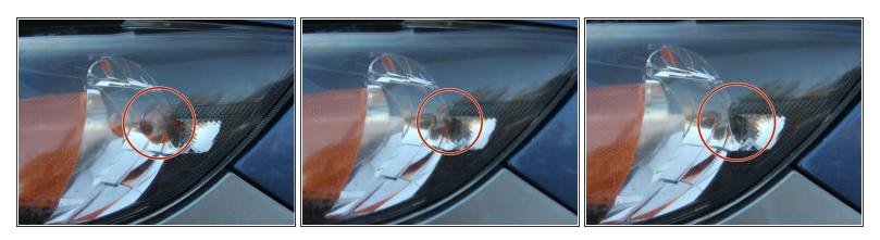
You should see the bulb being removed from its front-turn signal location.
