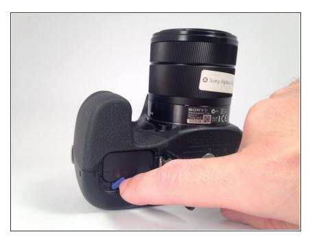
Push back the blue tab releasing the battery which should spring forth on its own.
