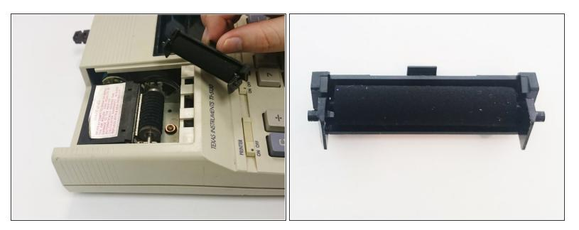
Pull up on the cartridge to remove it.
