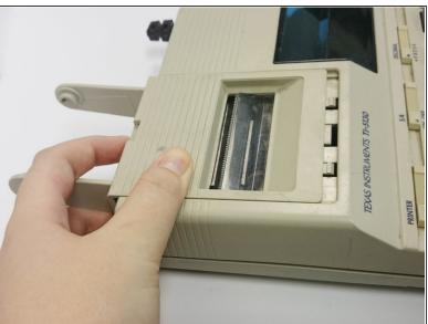
Remove the cover over the printer unit by pulling back on the cover.
