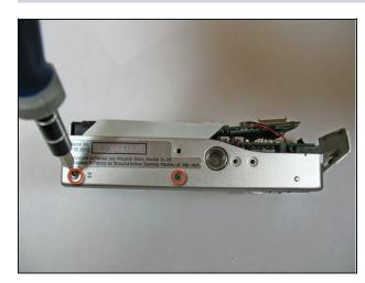
Remove the last two 2.8 mm Phillips #00 screws from the bottom of the camera.
