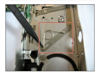
• Check the "V" shaped spring to see if it is connected to the body of the camera.
