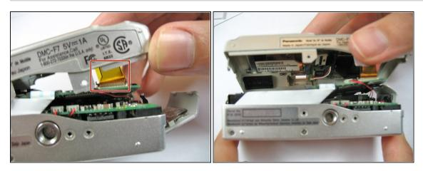
Be careful not to damage the ribbon cable when opening. Ensure it is still attached.
