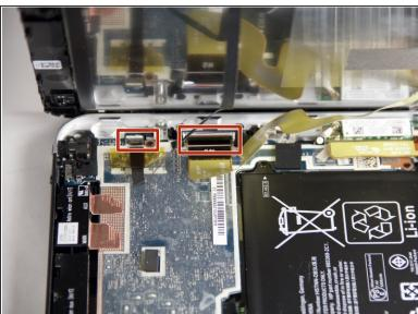
• Use the tip of a spudger to disconnect the two display **ZIF** connectors.
