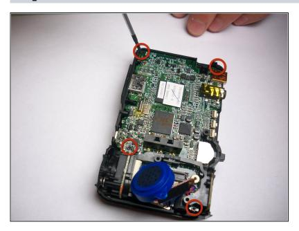
Remove the four Phillips head screws attaching the motherboard to the housing.
