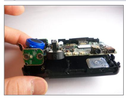
Using care, lift the motherboard from the plastic housing.
