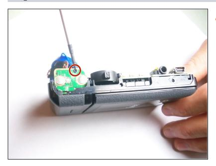
• Remove the individual 4mm screw under the top button to release the motherboard from the housing.
