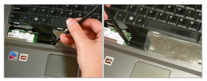
• Use a spudger to release the ribbon cable from the motherboard.
