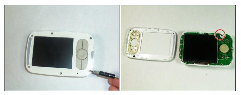
• Remove the four corner screws, 5.0 mm, using a J1 bit.
