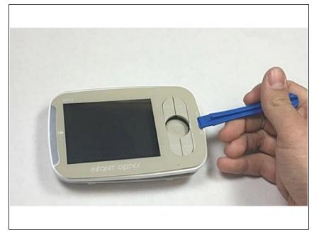
• Glide the tool around the entire cover to reveal the screws, which are 5.0 mm.
