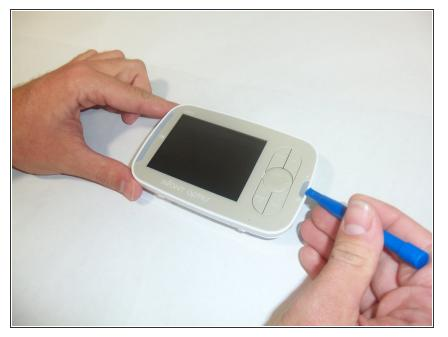
Start by gently inserting the plastic opening tool between the led and casing.
