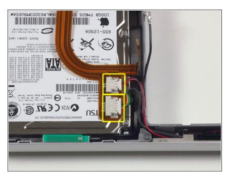
Disconnect the sleep light and IR sensor cable from the orange hard drive ribbon cable.
