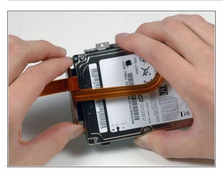
Lift the hard drive out of the computer and disconnect the orange ribbon cable from the drive.
