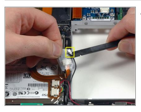
Lift the Bluetooth board out of its slot next to the hard drive and use a spudger to disconnect the Bluetooth antenna cable.
