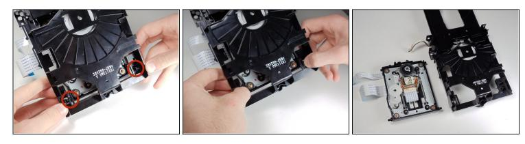
• Use your fingers to pull the shown tabs towards the sides of the tray, releasing the internal tray that contains the laser.
