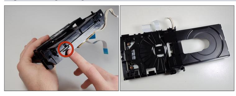
• Spin small gear shown right to begin opening the tray. There should be relatively little resistance in the gear.
