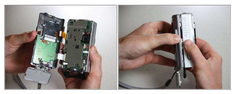
• Carefully slide both halves of the camera together, making sure all tabs are aligned. Press the sides firmly together until you hear a click.
