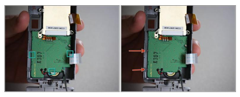
• Use the *plastic opening tool* to carefully pry the motherboard out of its place, proceeding from the indicated points. Pull gently, as to not destroy any of the other internal parts of the camera.
