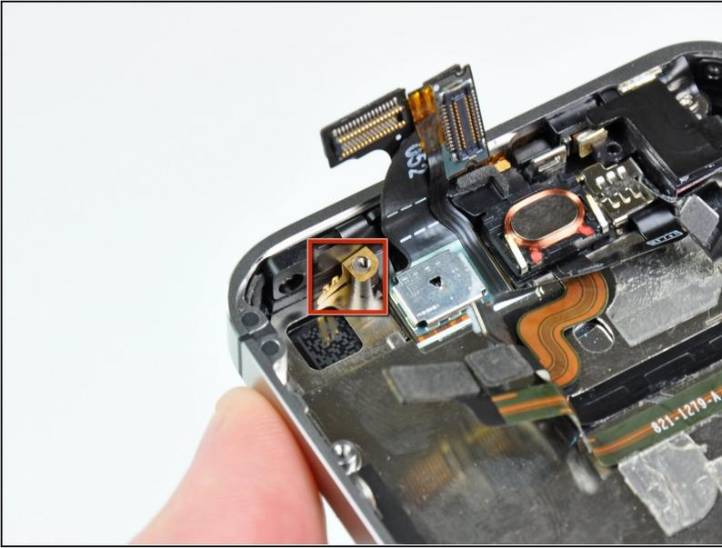
⚠ Be sure not to lose the small grounding finger for the rear facing camera near the power button.
