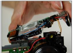
• With the lens facing towards you, pull the L-shaped frame away from the camera.
