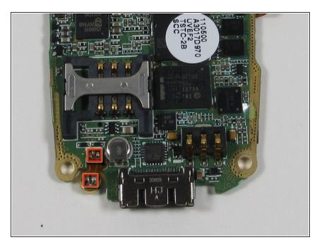
Solder joints are accessable to replace the microphone.
