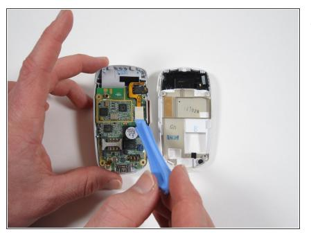
• Remove the ribbon wires connecting to the screen using the pry tool.
