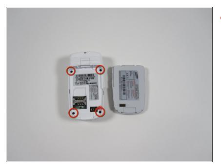
Remove the 4 (4.7mm) philips head screws.
