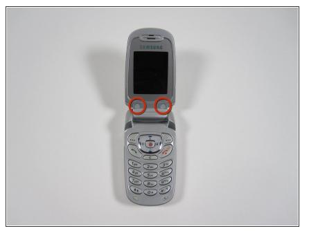
First, remove the 2 silver stickers (as indicated by the circles) with a a safety or push pin to reveal 2 screws.
