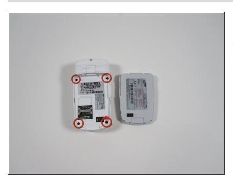
Remove the 4 (4.7mm) philips head screws.
