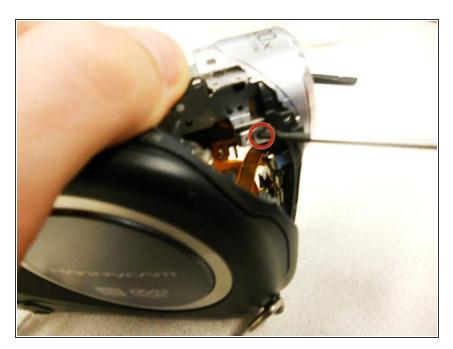
Remove the 4.5 mm screw that connects the camera body to the lens on the DVD side of the camera.
