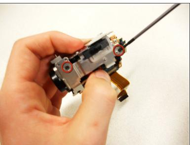
Unscrew the three 2.9 mm black screws to remove the metal bracket from the lens.
