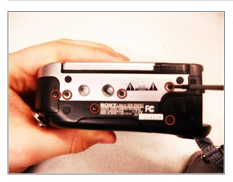
Using a #00 Phillips screwdriver, remove the six 4.5 mm screws from the camera's bottom.
