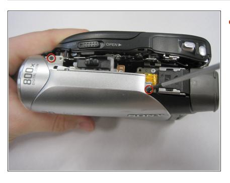
Remove the two 2.9 mm screws under the black plastic casing.
