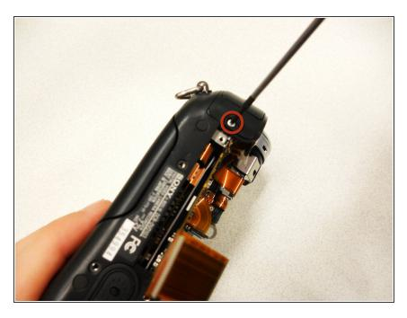
Remove the 4.5 mm thread that connects the lens to the camera body.
