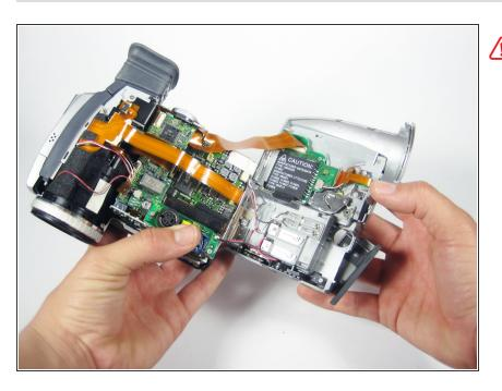
The side of the device should now be open as shown. Again, there are wire connections between the side cover and the body of the camcorder. Do not separate the two entirely!
