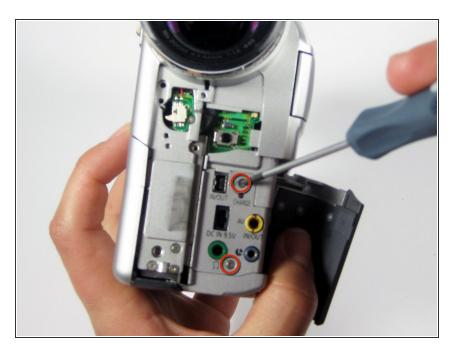
Remove 2 Philips #00 4mm screw shown.
