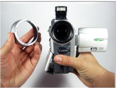
To remove the camcorder lens hood, twist the hood to counterclockwise and it will come loose, then pull towards you.
