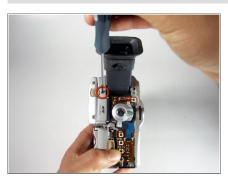
Remove the 4mm #00 Phillips screw located to the right of the LCD release switch.
