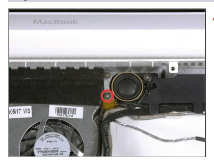
If you didn't remove the ground lug retaining screw in step 20 above, remove it now. It's a 7mm (may be 4mm or 3mm in Santa Rosa/Penryn and 2009 models) Phillips screw securing the ground lugs on the right speaker cable and microphone cable to the metal frame.
