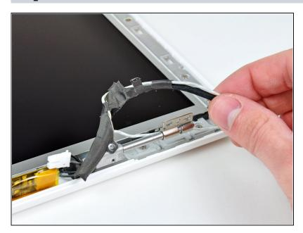
Move the display data cable out from under the mounting arm of the right clutch hinge.
