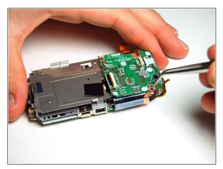
• With the tweezers, carefully peel back the copper ribbon that was underneath the black screw.
