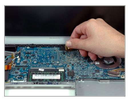
Peel up the orange Kapton tape securing the right thermal sensor cable to the logic board.
