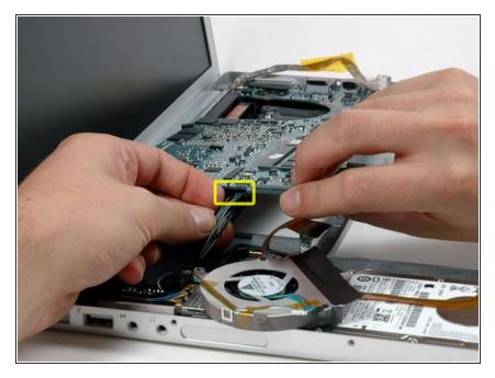
Lift up the left side of the logic board and disconnect the gray and black power cable from the bottom of the board.
