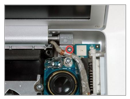
Remove the silver T6 Torx screw securing the ground loop in the display data cable to the casing.
