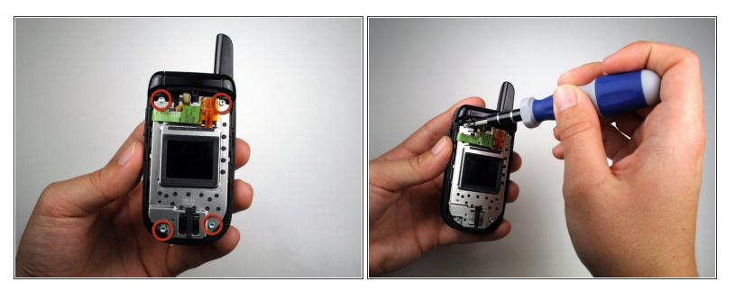
• Remove the four 5mm screws on the metal casing using the T6 Torx screwdriver.
