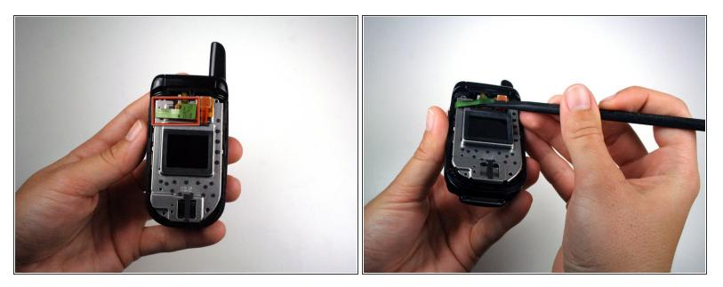
• Using the spudger, disconnect the green display cable.
