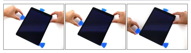
• Slide the left-hand opening pick down the edge of the display until you reach the corner.
