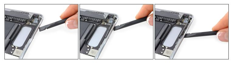
• Using a spudger or your finger, press in on the volume buttons to pop out the button component board.
