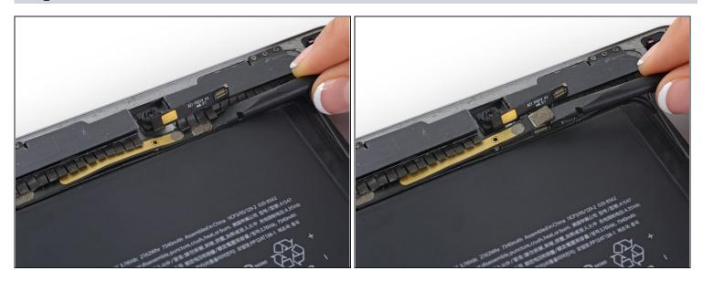
• Disconnect the headphone jack cable connector from its socket on the logic board.
