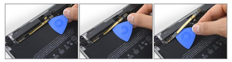
• Slide an opening pick under the headphone jack ribbon cable to free it from the adhesive securing it to the rear case.
