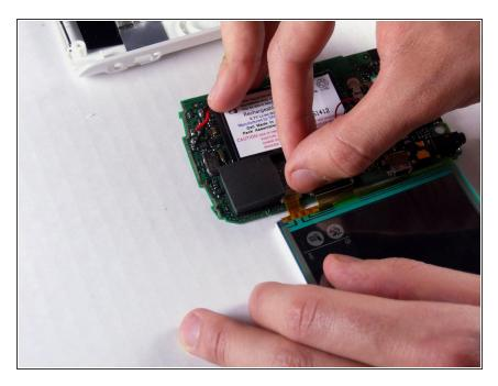
Carefully pull back the brown cable holders and separate the screen from the motherboard.
