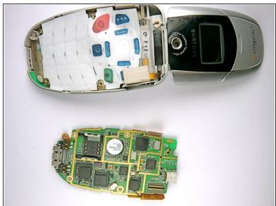
Detach the motherboard by grabbing the edges of it and lifting it straight out of the phone.
