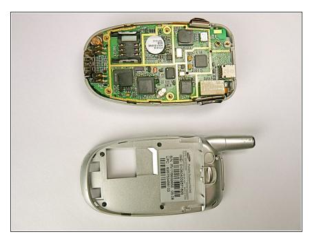
With the back panel removed, the motherboard should be fully exposed.
