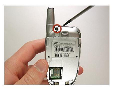
Unscrew the 4.5mm screw located underneath the rubber cover.
