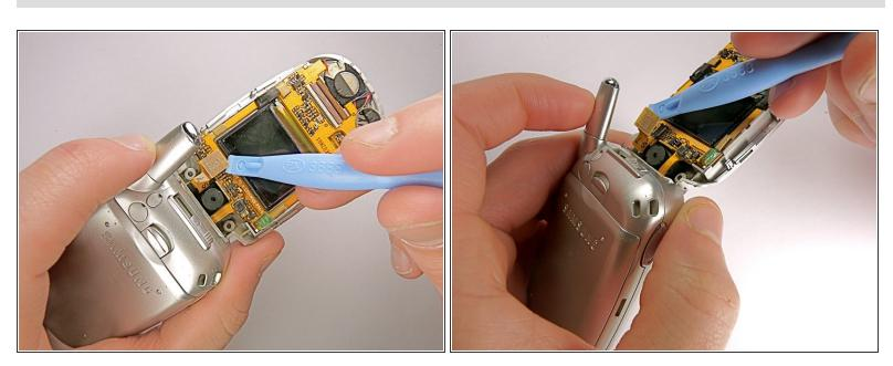
Detach the connecting wire panel from the LCD display system.
