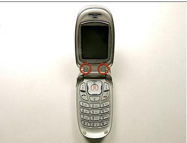
Remove the plastic coverings at the base of the LCD screen using your fingers.
