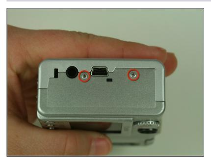
On the side of the camera, remove the two 4.75 mm screws that sit near the USB digital terminal.
