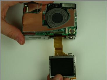
• Remove the LCD screen and set it aside.
