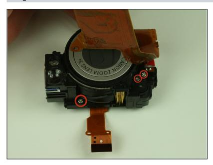
Remove the three 2.5mm screws underneath the flex circuit.
