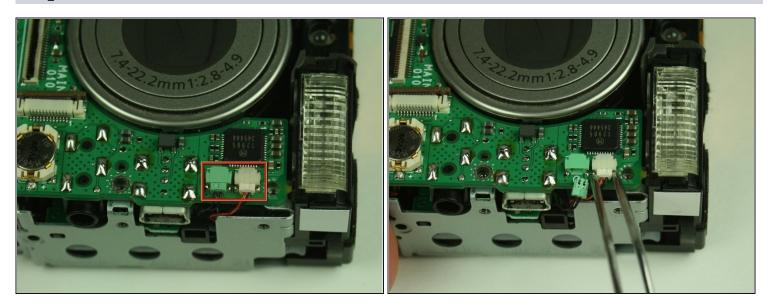
• Detach the white-capped and green-capped wires, which sit near the flash.
