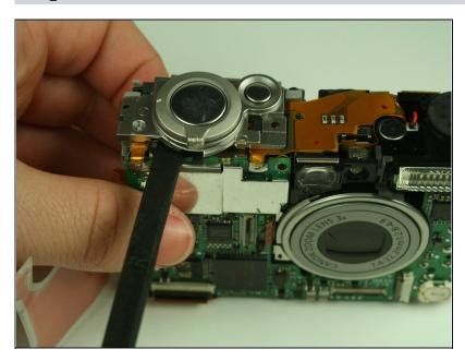
Using a spudger, gently detach the shutter button assembly from the camera.
