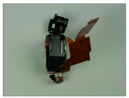
• Remove the small 1.5mm screw attaching the metal plate to the lens assembly.
