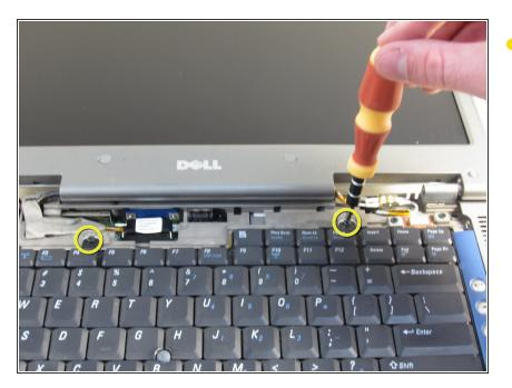
Remove the two 3mm screws on the top of the keyboard (nearest to the screen)
