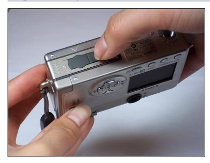
On the bottom of the camera, use your thumb to press the rubber battery cover towards the side of the camera with the strap base. The cover will shift to extend beyond the rest of the camera.
