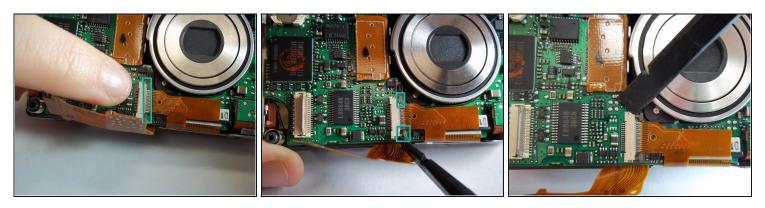
• Release the ZIF connector securing the next ribbon cable. To do this, insert the flat end of a spudger between the dark brown piece and the white piece of the connector. Since the dark brown piece is under the ribbon cable, move this piece to the right by wedging one end at a time.
