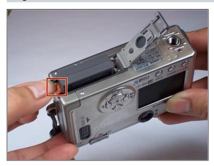
Locate the orange tab next to the battery. Next roll the tab back in order for the battery to come out.
