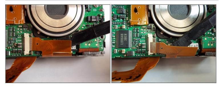
• Insert the spudger under the ribbon cable and gently pull the cable out of its port.
