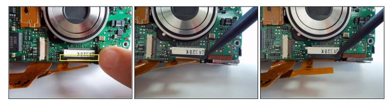
• Release the ZIF connector securing the ribbon directly below the lens. To do this, insert the pointed end of the spudger between the black piece of the connector and the white piece. Wedge the black piece down.
