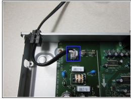
Take out the two ribbon cables adjacent to the DVD drive and the power supply in the upper left hand corner of the board (with the DVD drive oriented on the right) before attempting to remove the main board.
