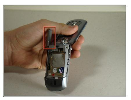
• Locate the antenna port on the top of the phone.
